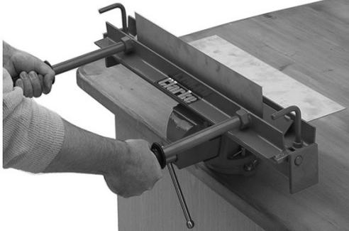
A metal folder held in a bench vice, showing a hand using a tool to fold a sheet of metal. |
